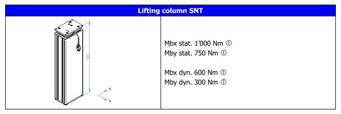
① Mb stat. = static bending moment = max. allowed bending moment while standstill Mb dyn. = dynamic bending moment = max. allowed bending moment during lifting movement
