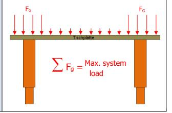
\* It is not allowed to place the max. load onto the table in a fast motion (crane or lift truck)!
