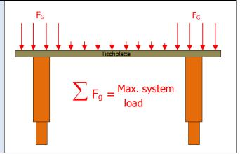
It is not allowed to place the max. load onto the table in a fast motion (crane or lift truck)!
