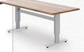
The base frame **SM-4** consists of four lifting columns arranged in a rectangle and connected by crossbars. The lifting columns are equipped with a foot plate including adjustable rubber feet. The table top is attached directly to the adapter plates of the lifting column **SM**.
